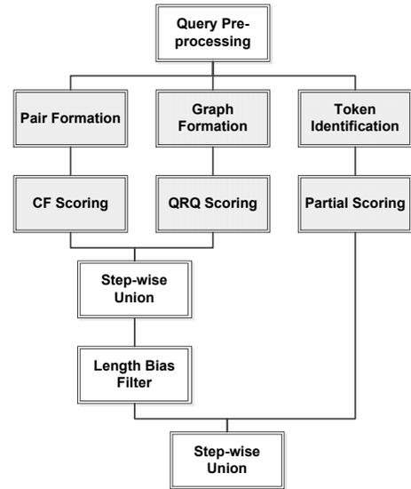
**Figure 4: Dataflow in the Metaphor pipeline. Each stage consists of one or more MapReduce jobs that process loaded query and click data.**
