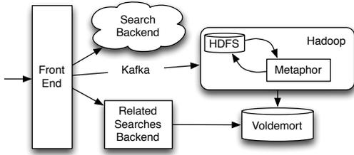
**Figure 3: Dataflow in LinkedIn's production system. Tracking data is aggregated through Kafka, and after processing the data in Hadoop, related searches recommendations are stored in Voldemort to serve to end users.**
